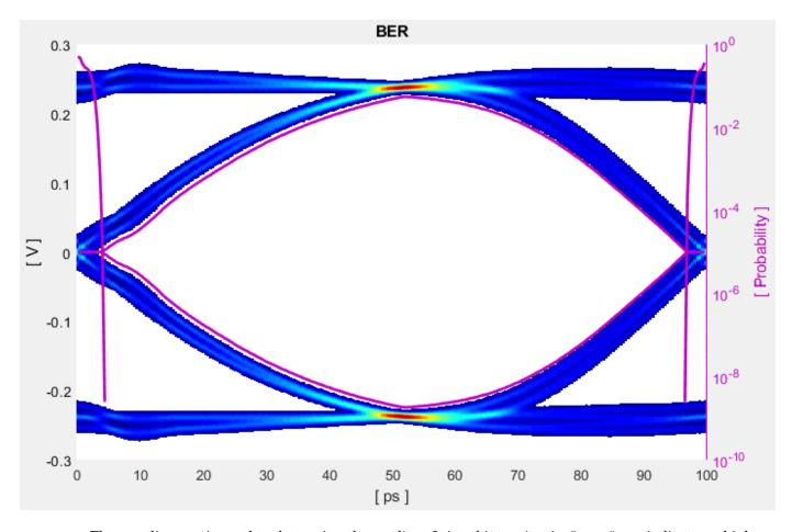
The eye diagram is used to determine the quality of signal integrity. An "open" eye indicates a higher probability of bit recovery. The bathtub curve plots the bit error rate as a horizontal function of the data eye and corresponds to eye width. The contour curve plots the bit error rate as a vertical function of the data eye, and corresponds to eye height.
